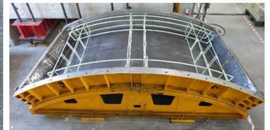
Tunnel segment GFRP reinforcement Meda et al. «Hybrid precast tunnel segments in fiber reinforced concrete with glass fiber reinforced bars»
