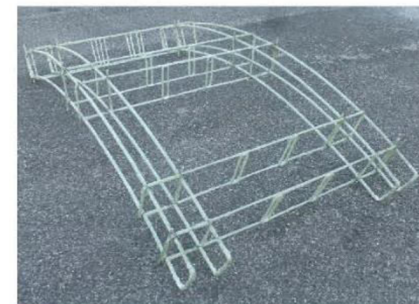
Tunnel segment GFRP reinforcement Meda et al. «Hybrid precast tunnel segments in fiber reinforced concrete with glass fiber reinforced bars»
